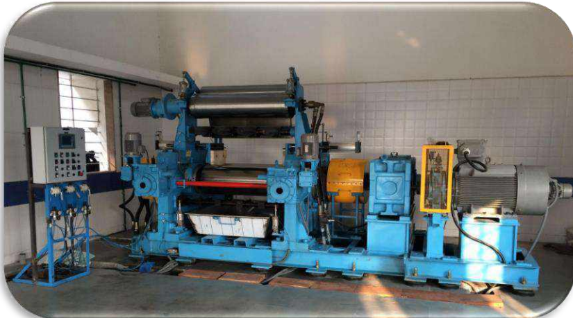
Mixing Mill with Peripherally Drilled Rolls & Stock Blender (Make: Bainite)
